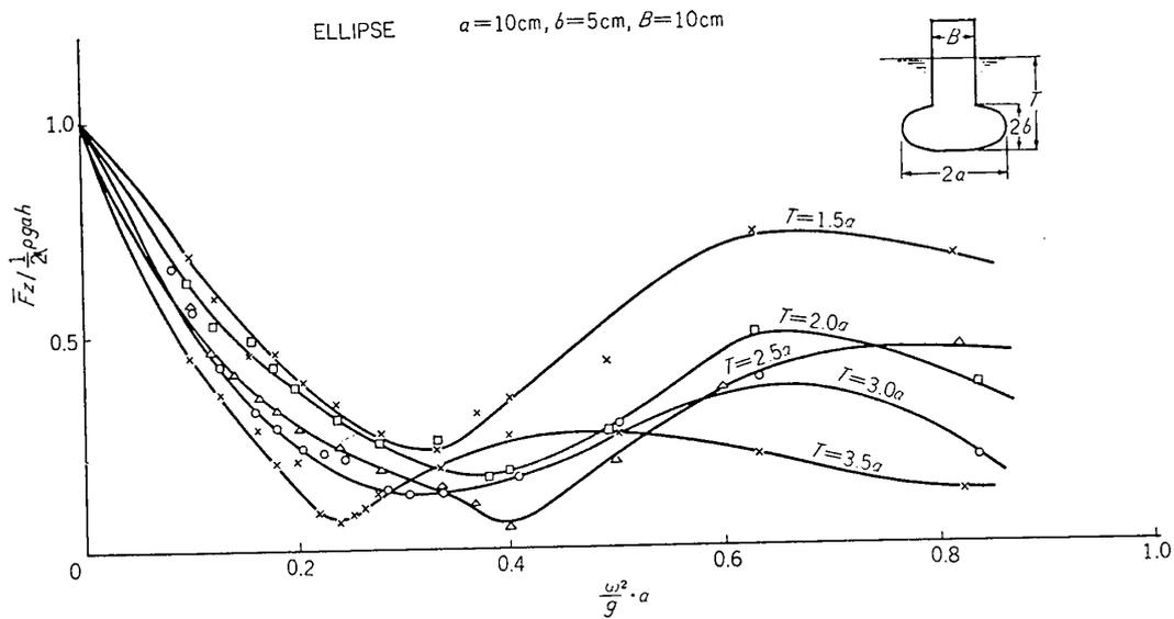
Fig. 9 a). Heaving force of elliptic cylinder type ( $a/b=2$ ).
