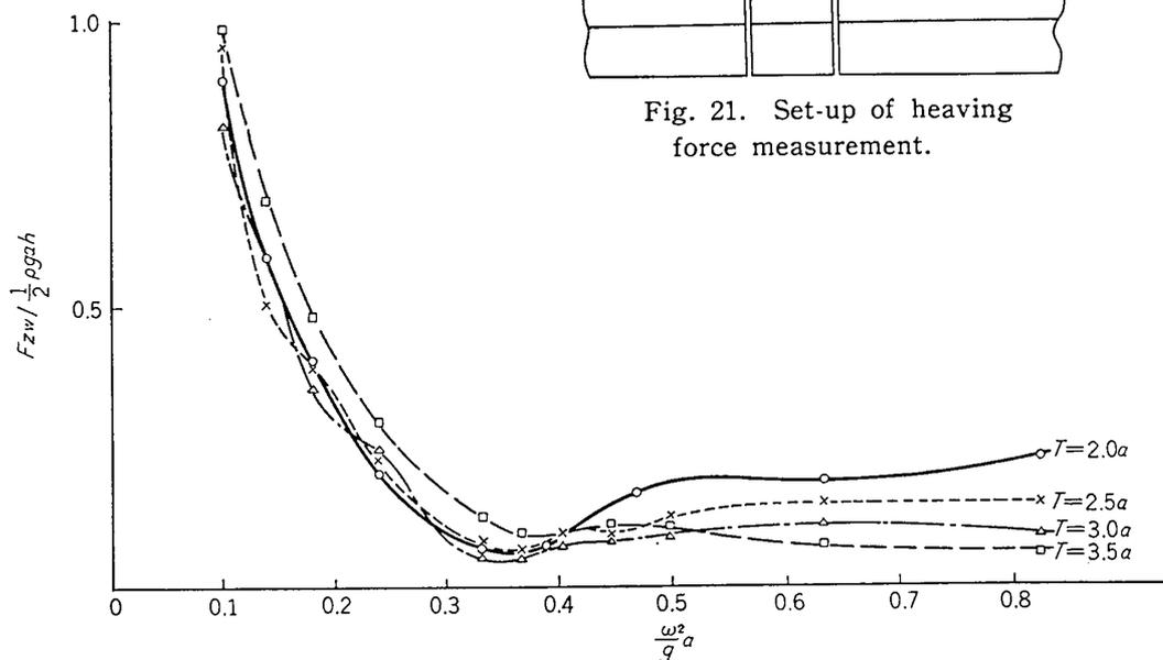
Fig. 22. Heaving force per unit length of an elliptic type prism in longitudinal wave.
