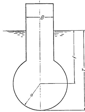
Fig. 1. Geometry of circular cylinder type models.
