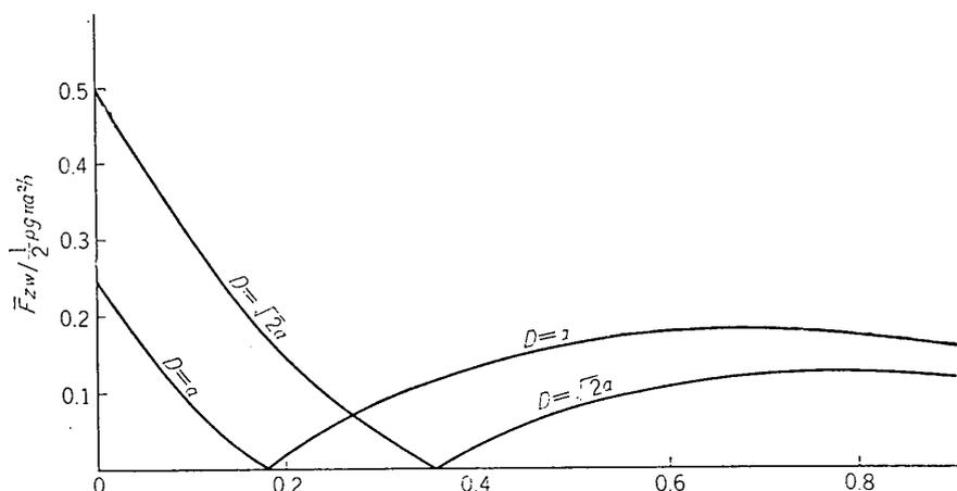
Fig. 18. Calculated heaving force of sphere type models.
