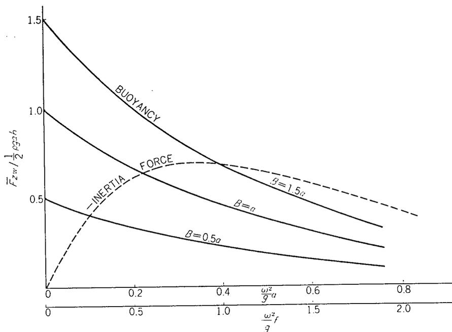
Fig. 2. Calculated inertia force and buoyancy for different breadth of the strut.
