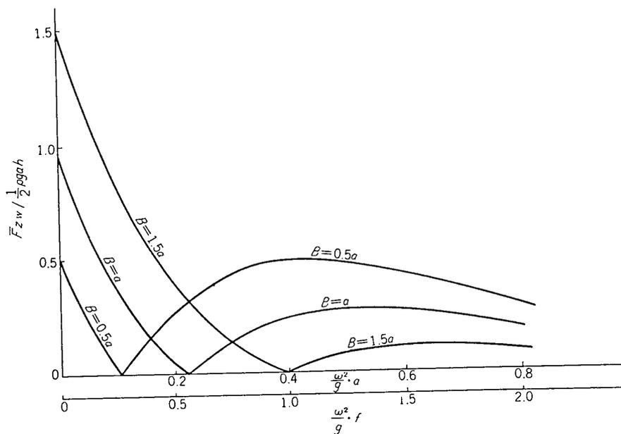
Fig. 3. Calculated heaving force of circular cylinder type models.
