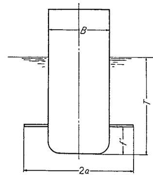
Fig. 10. Geometry of fin type models.
