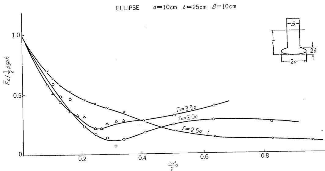
Fig. 9 b). Heaving force of elliptic cylinder type ( $a/b=4$ ).
