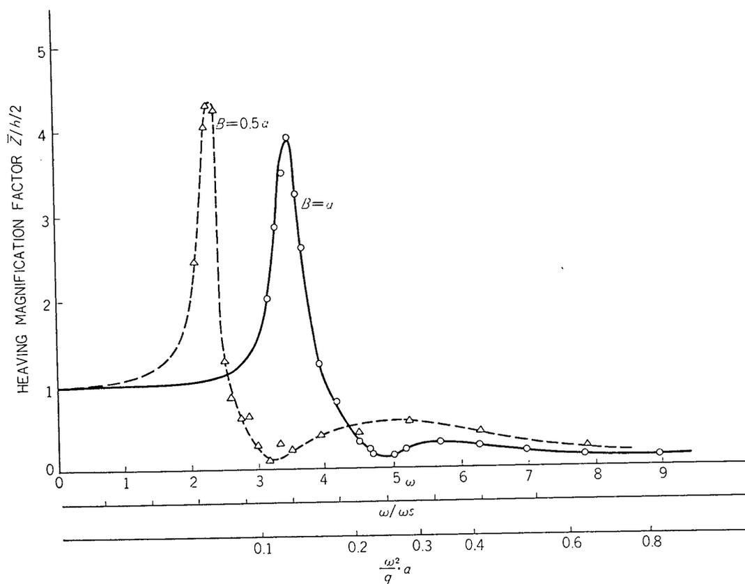
Fig. 12. Heaving magnification factor of circular cylinder type model.
