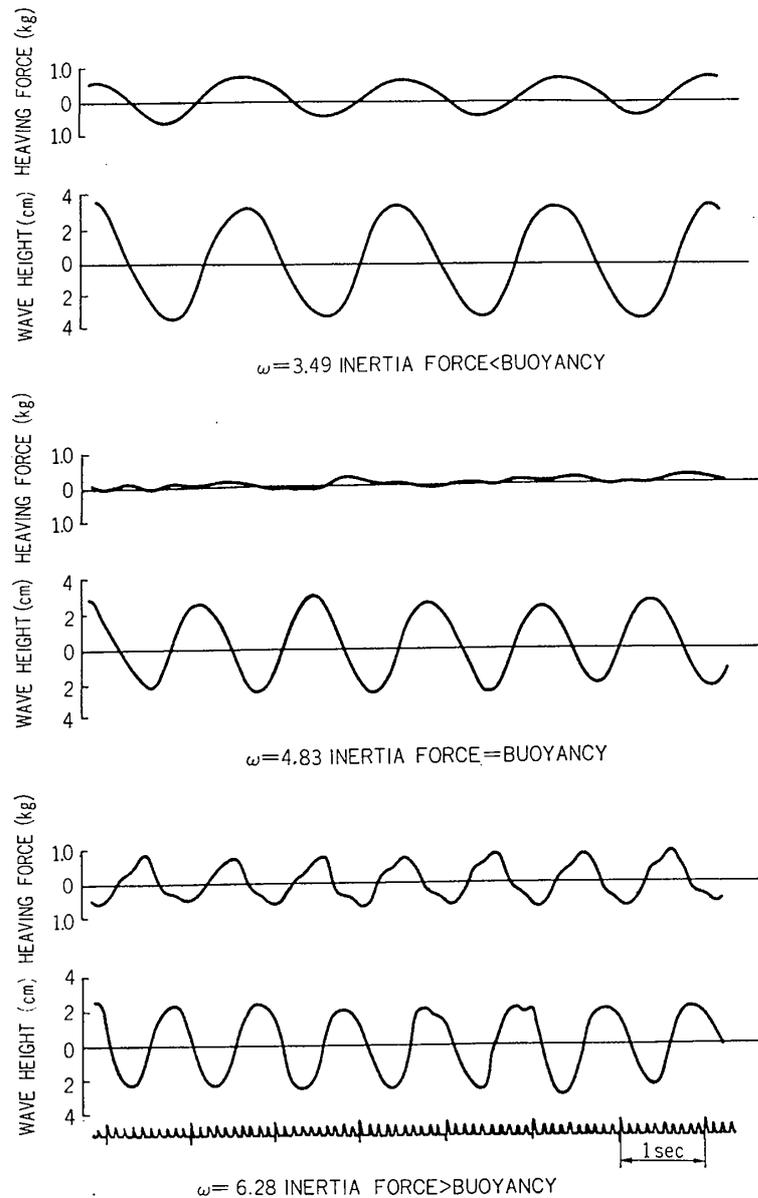
Fig. 6. Typical oscillogram of the heaving force and wave elevation.
