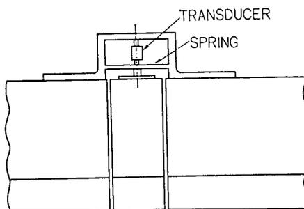
Fig. 21. Set-up of heaving force measurement.
