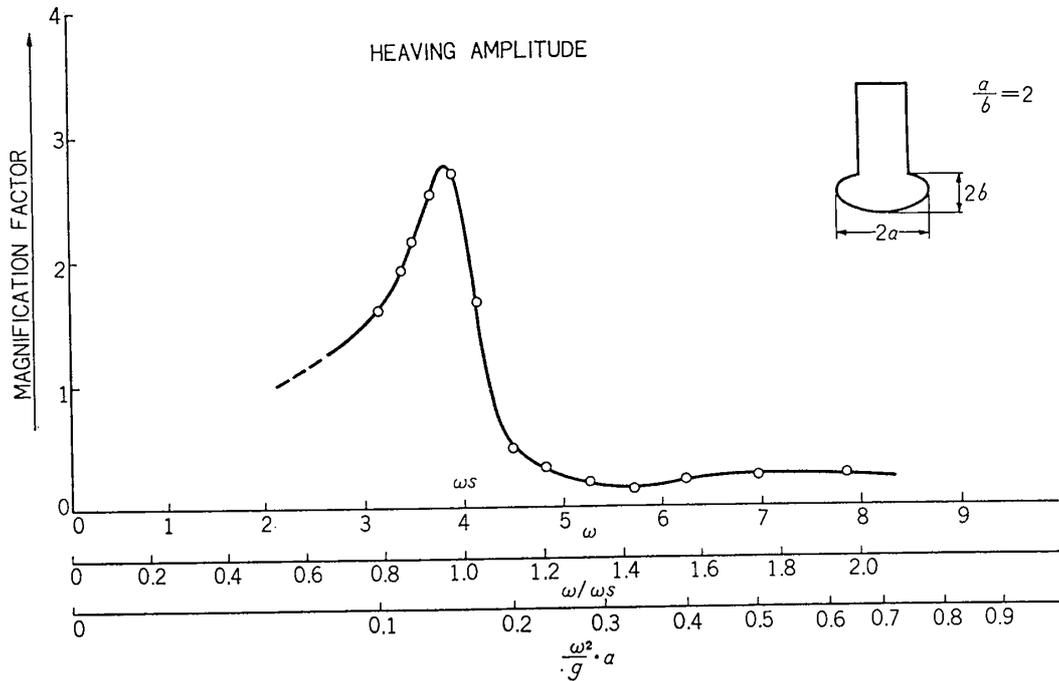
Fig. 13 a). Heaving magnification factor of an elliptic cylinder type model ( $a/b=2$ ).
