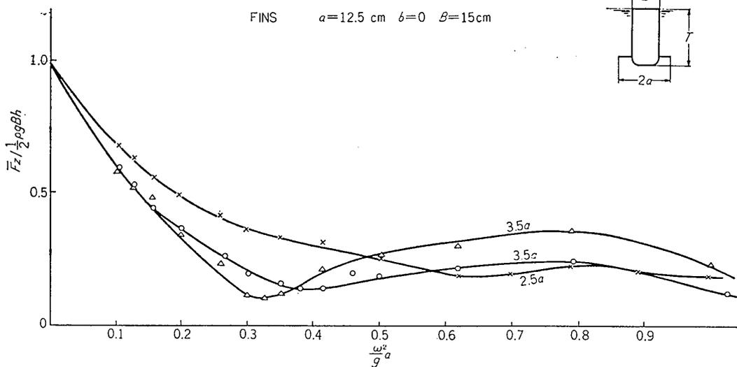
Fig. 11. Heaving force of fin type models.
