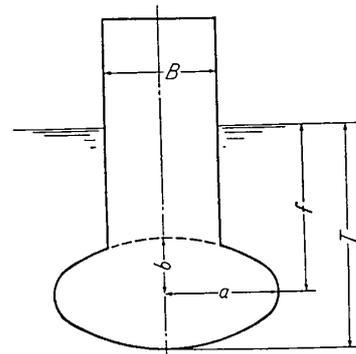
Fig. 8. Geometry of elliptic cylinder type models.
