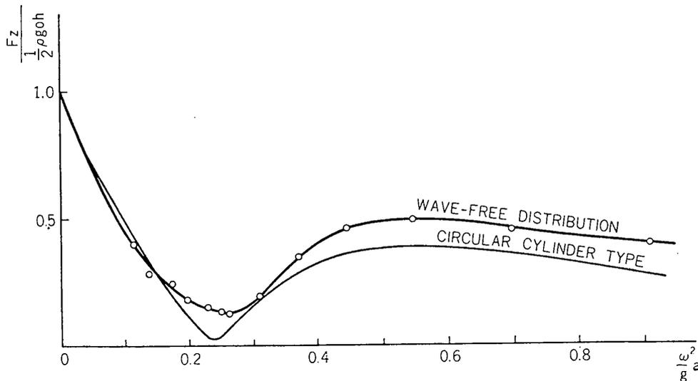
Fig. 25. Comparison between the heaving force of a wave-free body obtained by Bessho and that of the circular cylinder type model.
