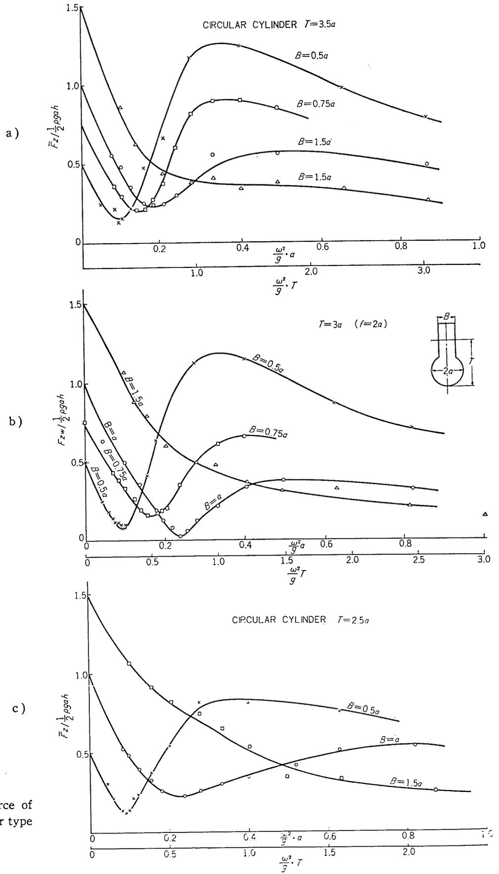
Fig. 7. Heaving force of the circular cylinder type models.
