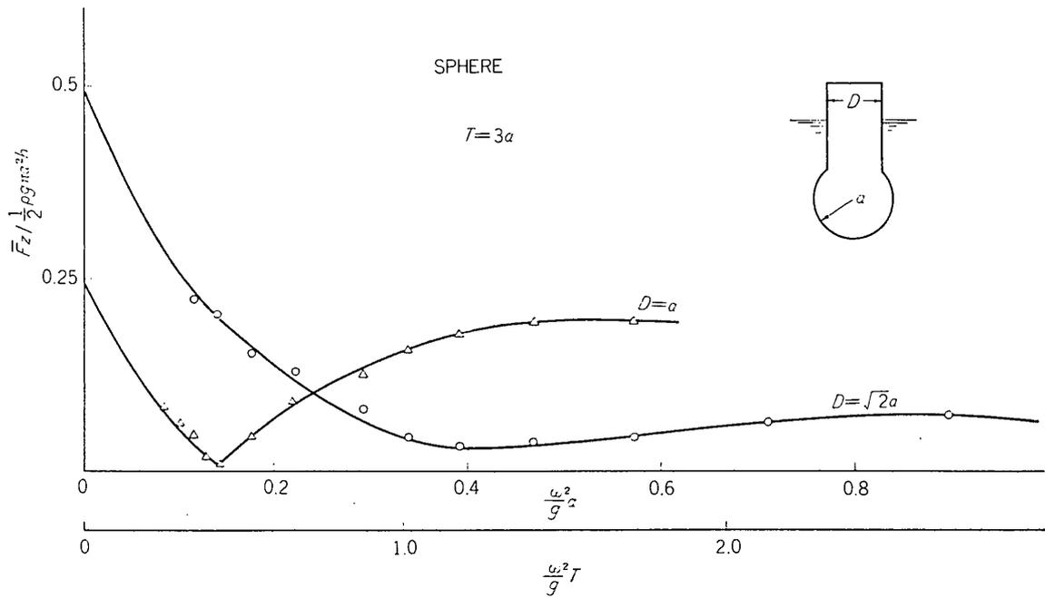
Fig. 20 b). Heaving force of sphere type models ( $T=3a$ ).
