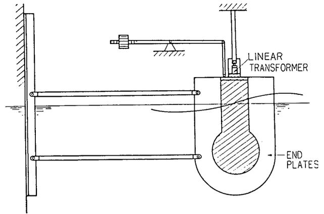
Fig. 4. Set-up of heaving force measurement.
