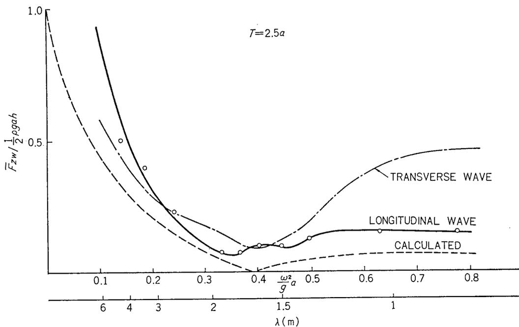
Fig. 23. Comparison of heaving force in longitudinal waves with that in transverse waves.
