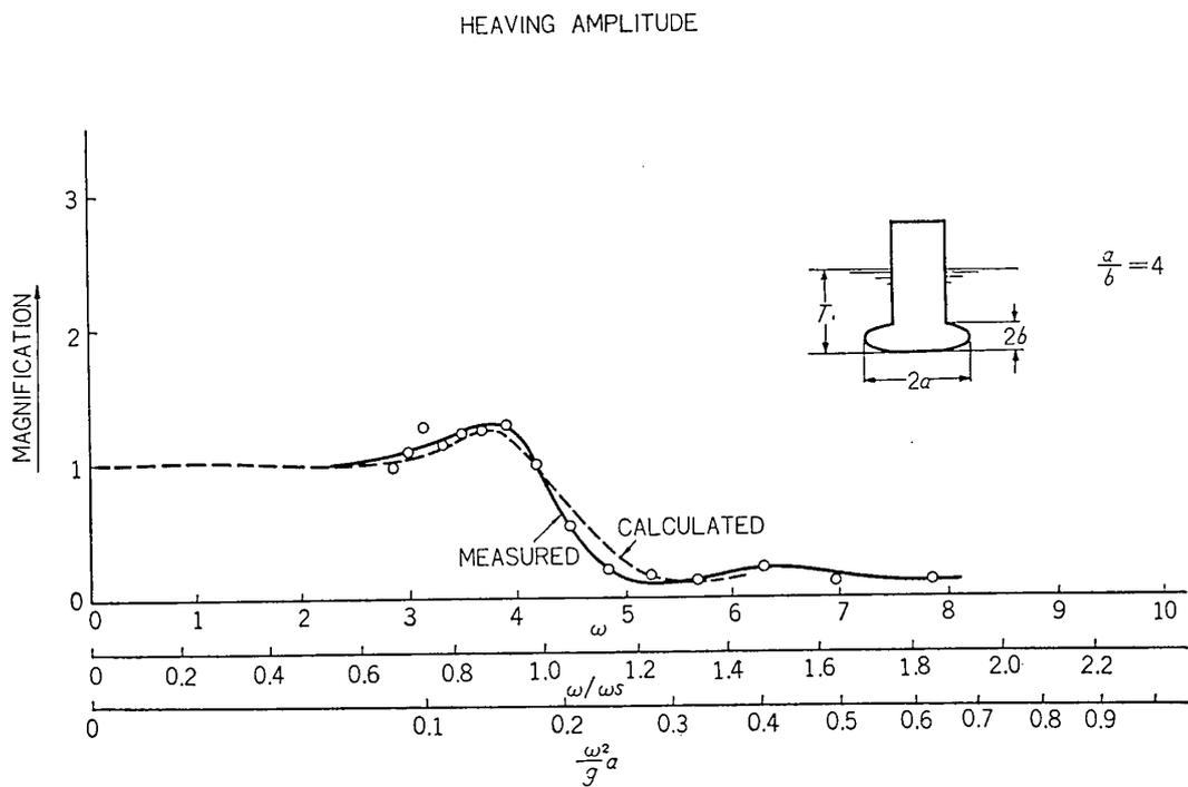
Fig. 13 b). Heaving magnification factor of an elliptic cylinder type model ( $a/b=4$ ).
