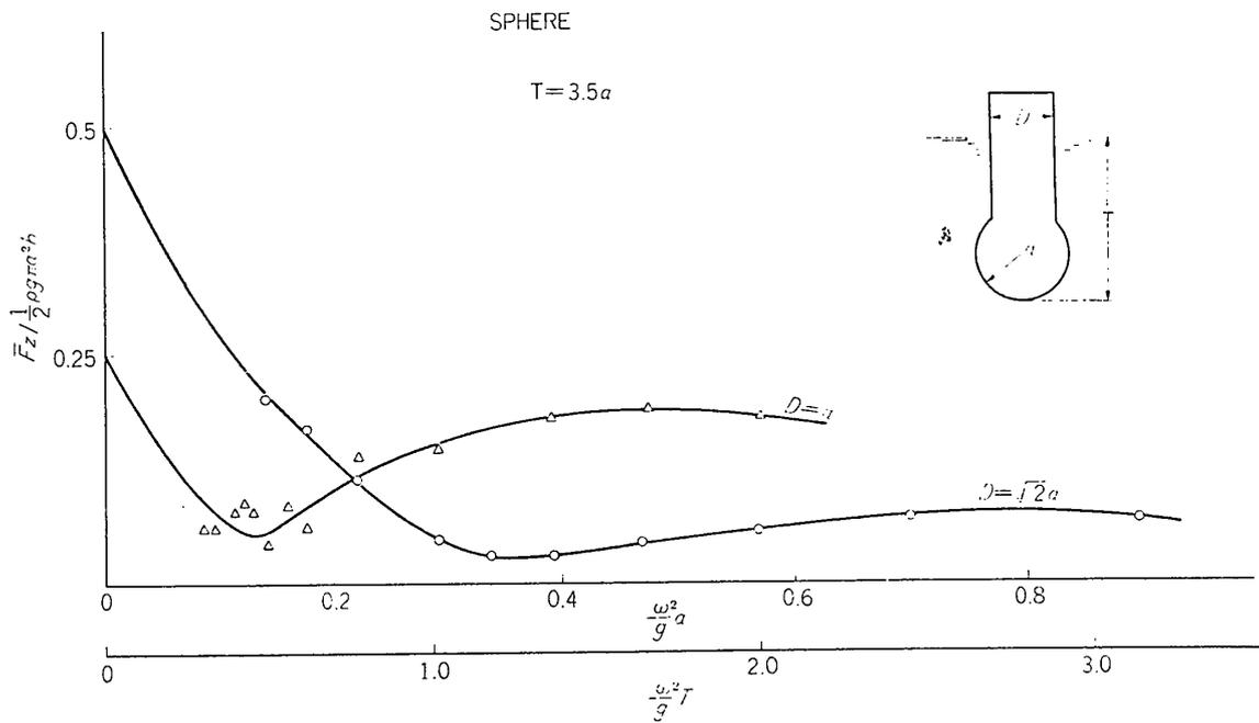
Fig. 20 a). Heaving force of sphere type models ( $T=3.5a$ ).
