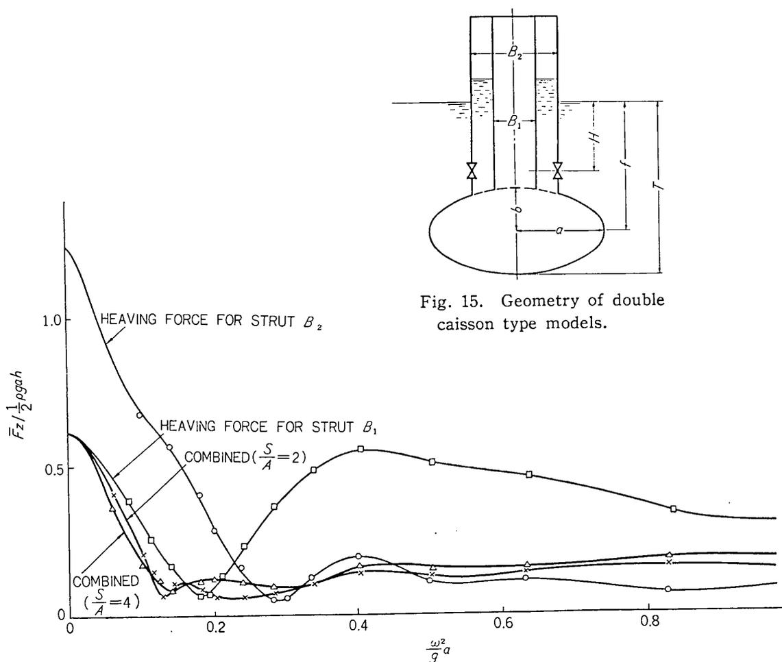
Fig. 15. Geometry of double caisson type models.
