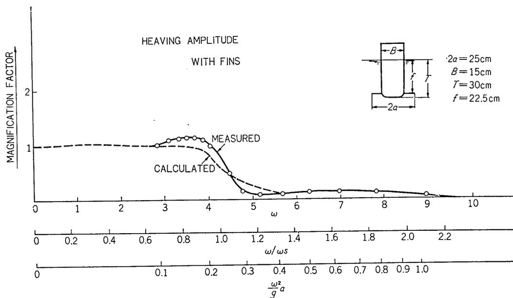
Fig. 14. Heaving magnification factor of a fin-type model.
