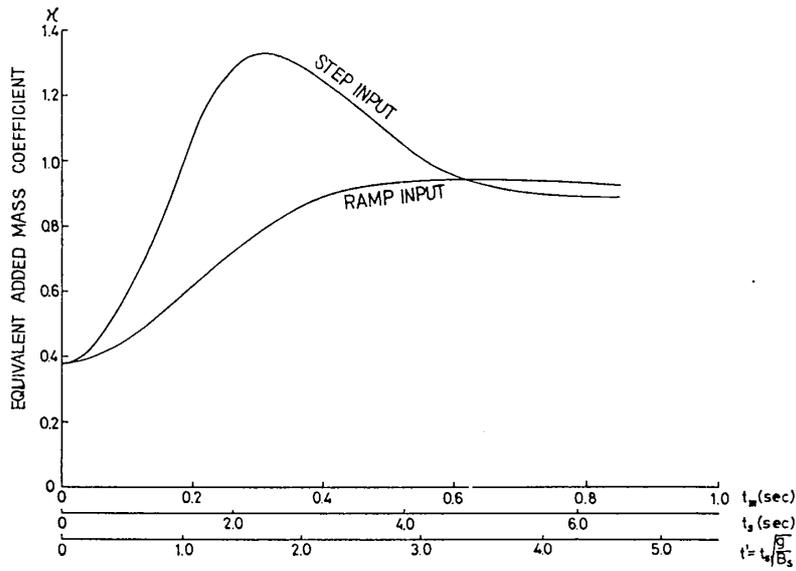
Fig. 3 Equivalent added mass  $\bar{m}_y''/m^*(=\kappa)$
