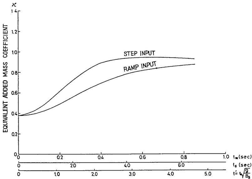
Fig. 4 Equivalent added mass  $\bar{m}_y'/m^*(=\kappa)$
