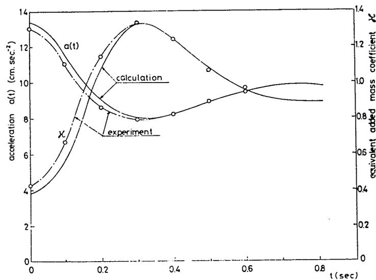
Fig. 7 Acceleration  $a(t)$  and equivalent added mass  $m_y''/m^*(=\kappa)$
