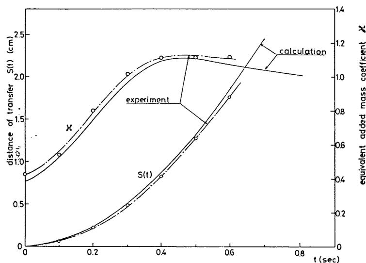
Fig. 9 Translation  $s(t)$  and equivalent added mass  $\bar{m}_y/m^*(=\chi)$
