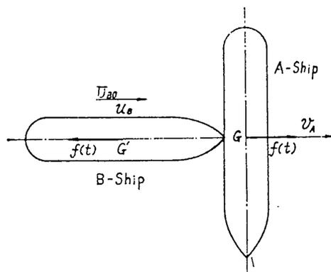
Fig. 10 Lateral Collision
