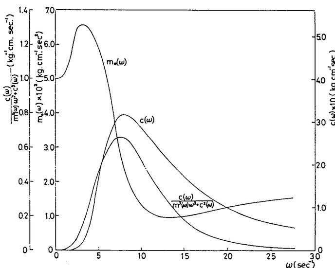
Fig. 1 Added mass  $m_0(\omega)$  and damping coefficient  $c(\omega)$  of the first atomic Ship of Japan at model scale
