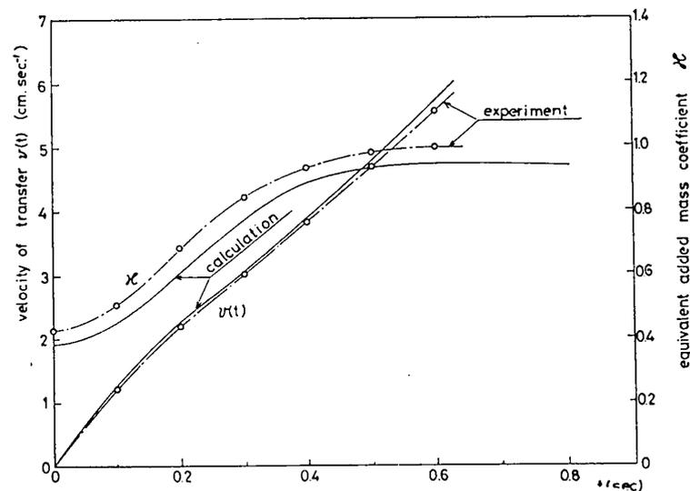
Fig. 8 Velocity  $v(t)$  and equivalent added mass  $\bar{m}_y'/m^*(=\chi)$
