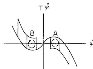
Fig. 5.5 Phase portrait with unusual moment which is symmetric with respect to the origin
