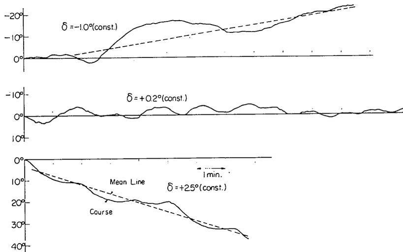
Fig. 2.7 Typical course record of spiral tests
