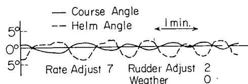
Fig. 2.2 Record of course and rudder angles when auto-pilot was used
