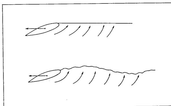
Fig. 6.5 Comparison of wakes of usual ship (upper side of figure) and ship affected with unusual moment (lower side)
