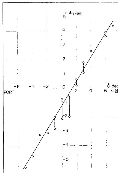
Fig. 3.1 Result of spiral tests (original model)
