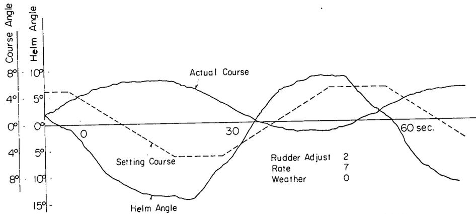
Fig. 2.4 Records of frequency response test by trapezoidal input
