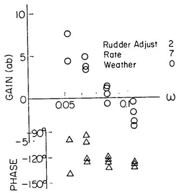
Fig. 2.5 Frequency response of loop transfer function
