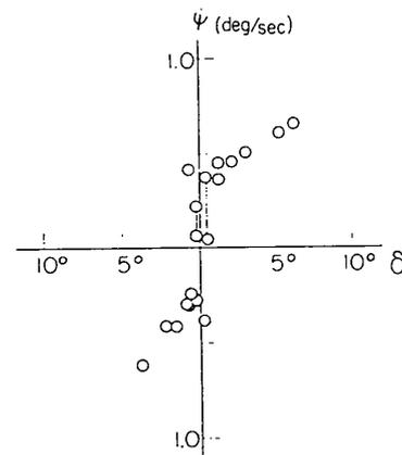
Fig. 4.2 Spiral tests of ship with fins
