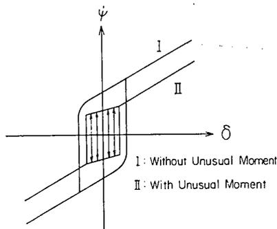
Fig. 5.3 Spiral test
