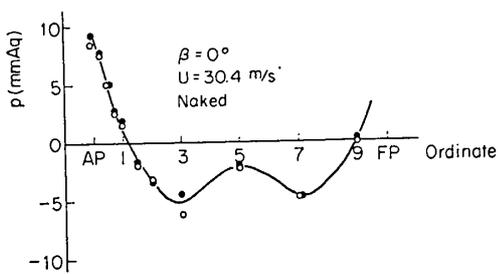
Fig. 6.2 (a) Pressure distribution around model ship (naked,  $\beta=0^\circ$ )
