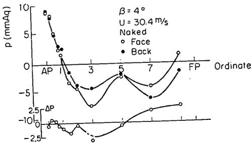
Fig. 6.2 (b) Pressure distribution around model ship (naked,  $\beta=4^\circ$ )
