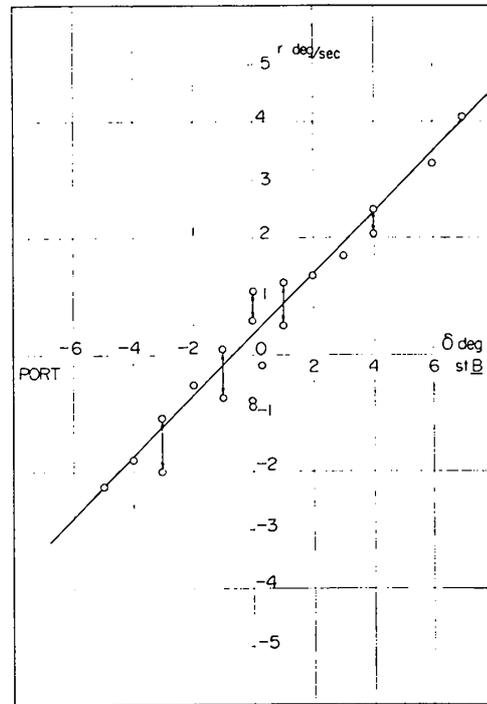
Fig. 3.5 Spiral tests (Fin No. 2)
